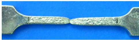
Fig. 3. Typical ductile failure mode of Sn–3.0Ag–0.5Cu solder.
